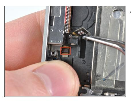
Remove the tiny rubber spacer near the dock connector.
