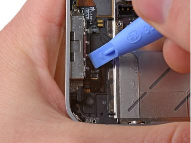
• Use a plastic opening tool to flip up the retaining flap on the home button ribbon cable ZIF socket.
