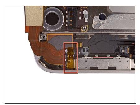
If present, remove the small strip of tape covering one of the dock connector screws.
