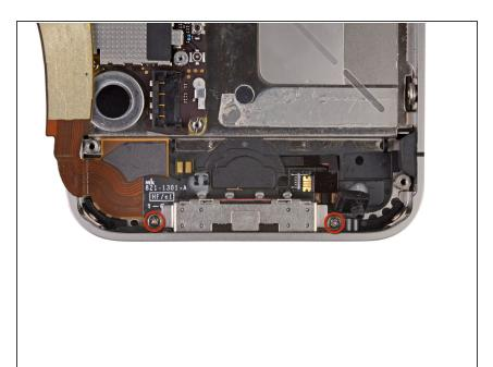
Remove the two 1.3 mm Phillips screws securing the dock connector to the case of the iPhone.
