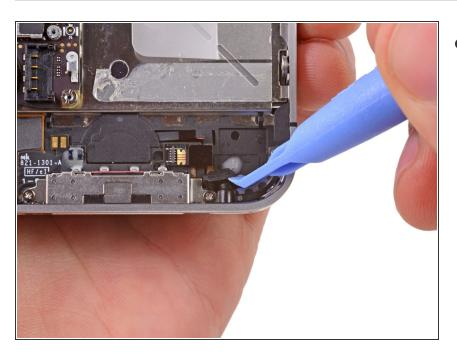
Carefully pull the rubber microphone holder out of its tube in the bottom edge of the iPhone.
